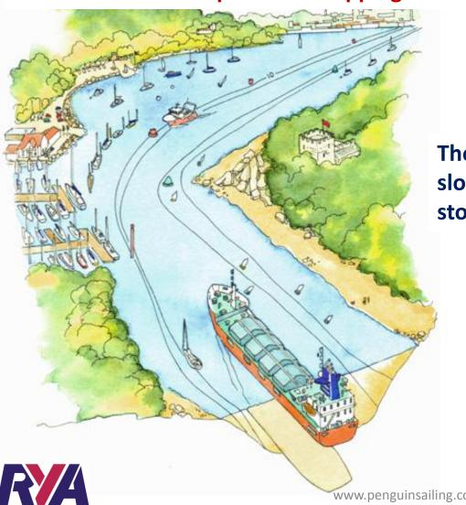
The ship has a large turning circle is slow to accelerate, decelerate and stop
