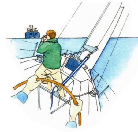
A hand bearing compass can be used to check the bearing
