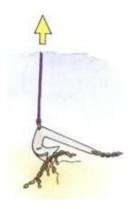
Raising a fouled anchor by the tripping line should clear the obstruction
