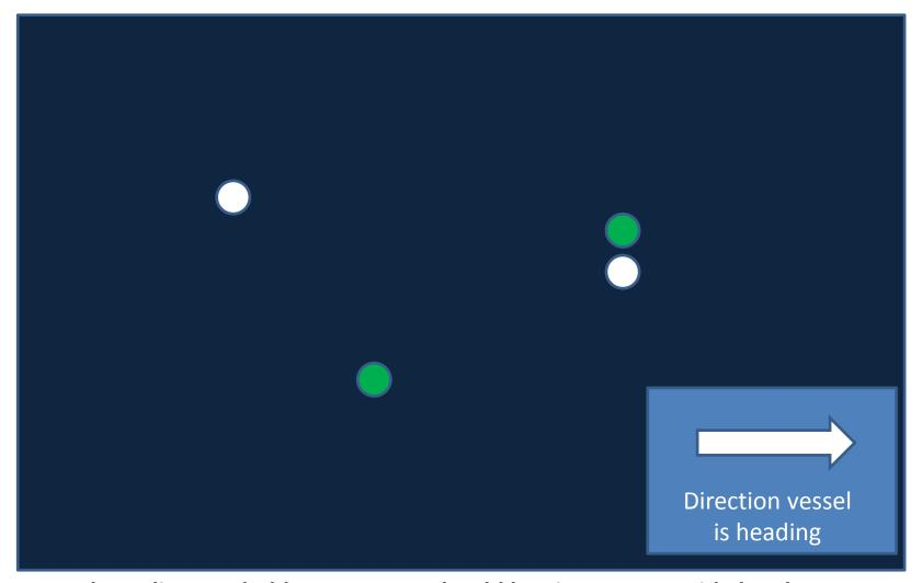
Vessel trawling, probably over 50m - should be given a very wide berth
