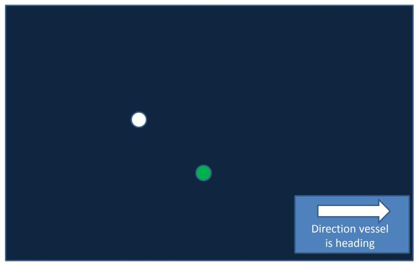
Sailing yacht with auxiliary engine on, ie, power driven vessel under 50m
