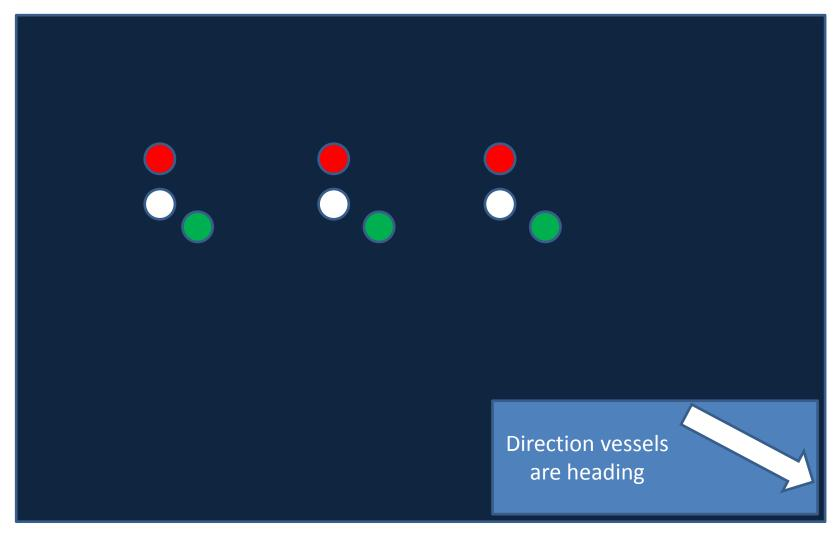
Three fishing boats - Starboard side Go round, rather than through, especially if it is a large fishing fleet
