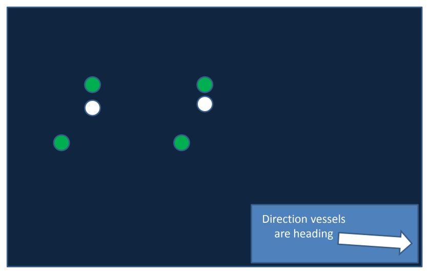
Trawlers engaged in pair trawling – starboard side You may also see the vessels shining search lights forwards and towards each other
