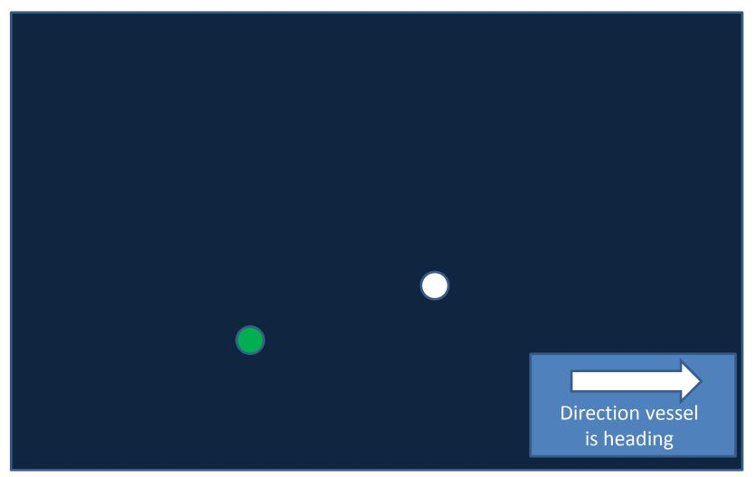
Power driven vessel under 50m
