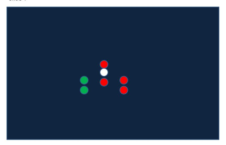
Working dredger not making way – pass on green side Two red lights on obstructed side – Two green lights on clear side Also shows lights for vessel restricted in manoeuvrability
