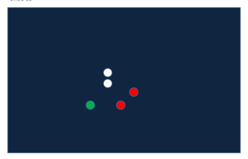
Tug and tow seen from ahead Two masthead lights show tug is towing Get out the way.....fast!
