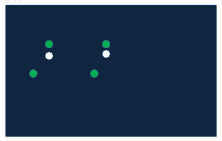
Trawlers engaged in pair trawling – starboard side
